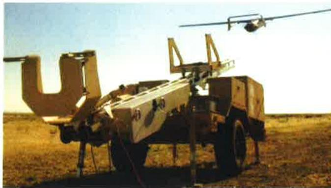
FIGURE 4-3: ARCTURUS T-20 PORTABLE CAPTURE SYSTEM
