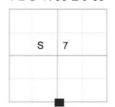
Set an iron post, 3 ft. long, 1 ins. diam., 26 ins. in the ground, for 1/4 sec. cor., with
