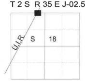
**DESCRIPTION OF CORNER EVIDENCE FOUND:** Found 2 1/2" iron pipe with 2 ½" GLO Brass Cap marked as shown below, protruding 15" above ground, from which:
