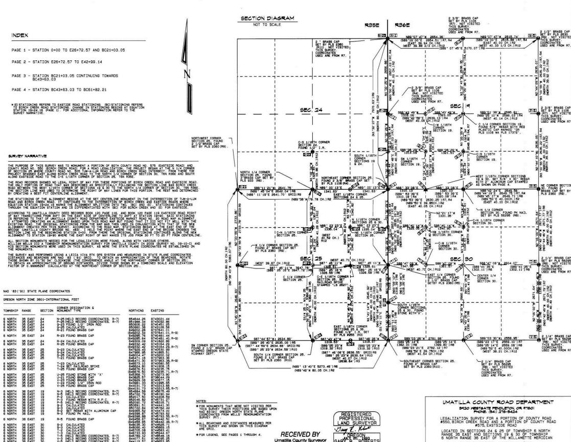
\*ALL BEARINGS AND DISTANCES MEASURED PER THIS SURVEY AND SHOWN ON THIS DIAGRAM ARE GRID.
